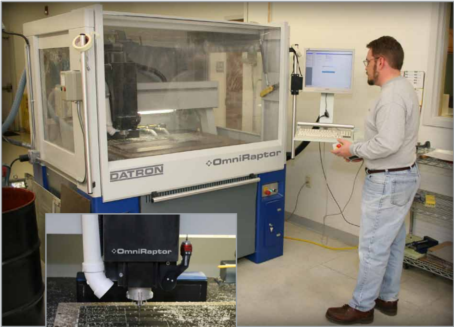
QC Drilling machine operator, Ron Twardosky, runs small flat Lexan parts on the DATRON M8 machining system — a run of 15 is not uncommon.
